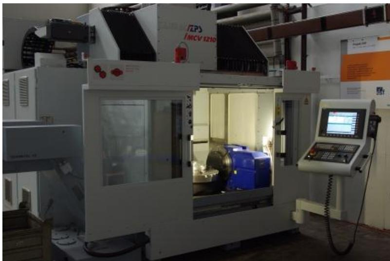
Fig. 6.1 5-axis machining centre MCV 1210 with the Sinumerik 840D pl
